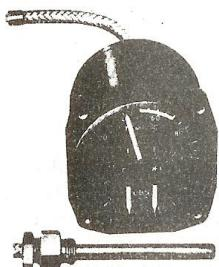
ENGINE GAUGE UNIT, Airomarine B-7 combines three indicating units, thermometer, oil pressure gauge and fuel pressure gauge, in one case. As these three engine instruments are ordinarily read together, they be quickly and easily checked when grouped in one case. The scales are so arranged that with normal operating conditions, the three pointers form an inverted "T", thus any change from this normal position is immediately apparent.
