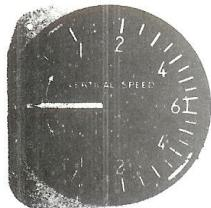
VERTICAL SPEED INDICATOR or " CLIMB " INDICATOR ( type A.N.5825-1 ) as it is frequently called, indicates the rate of change of the altitude of an airplane. It is used both as an aid to maintaining level flight and to indicate the correct speed of ascent or descent in taking off, landing or traveling through an overcast. The Vertical Speed Indicator operates with a connection to the static line of a pitot-static tube.
