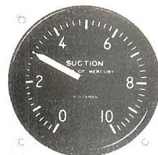
SUCTION GAGES (Kollsman) type 2650-A gives a continuous indication in inches of mercury of the suction being generated in a system. Kollsman Suction Gages are more sensitive than usual instruments of this type due to the use of a sensitive diaphragme as the actuating mechanism instead of the usual suction gages.
