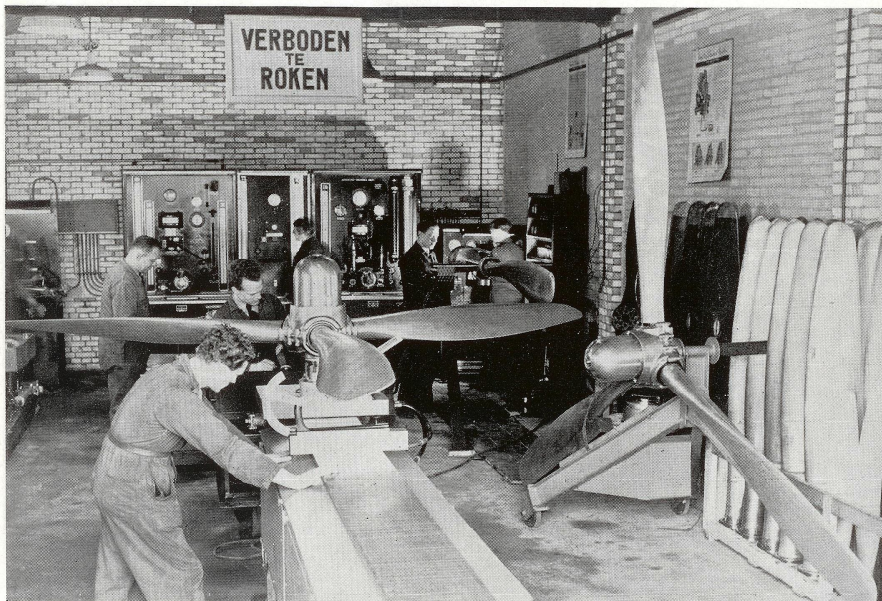
Propeller and accessory shop with modern equipment for testing carburettors, fuel pumps, hydraulic pumps, governors and other accessories.
